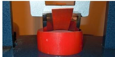
5. Remove the large radius anticlastic bracelet former and attach the small radius anticlastic bracelet former. Insert one end of the bracelet blank and press from the 20% mark to the end of the bracelet. Turn the bracelet around and press from the other 20% mark to the other end of the bracelet.
