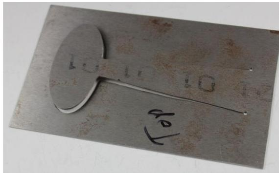
A blanking die, sometimes called a pancake die, is used for cutting multiple identical blanks during production work. The metal is placed in the blanking die and pressed in the hydraulic press causing the die to cut out the metal blank.
