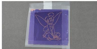
8. Hang the package on the edge of the tank by the strip of aluminum foil, and clamp it in place with the red alligator clip from the power supply. Add the electrolyte to the tank until it completely covers the metal blank, but do not allow the electrolyte to touch the aluminum strip or the alligator clip. Hang a copper cathode on the other side of the tank and connect it to the black alligator clip from the power supply.
