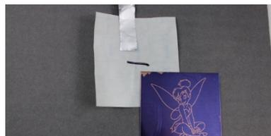
4. Remove the backing from the contact paper. Slip about half an inch of the aluminum strip through the slit from the non-sticky side to the sticky side, and stick the end of the aluminum strip to the sticky side below the slit. (For the photo, I set it down on the backing paper so it would not stick to my background.)
