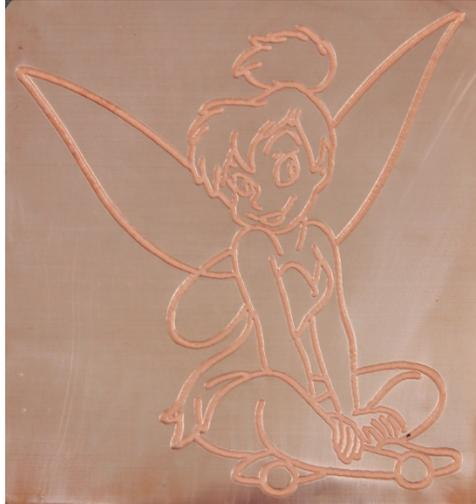
The positive space of the design will be etched into the metal and the negative space of the design will be left untouched above the design.
