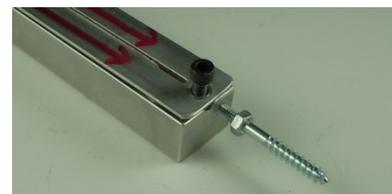
Screw the file handle onto the wood thread end of the hanger bolt.
