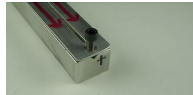
Using the #25 drill bit, drill a hole at least 1 inch deep into the left end of the Koil Holder.
