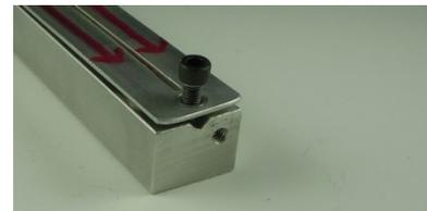
Apply oil to the tap and cut threads into the hole, all the way to the bottom.
