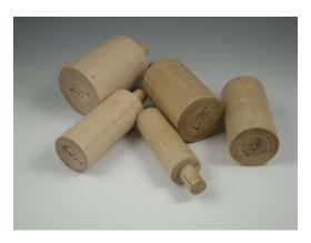
I had a friend make a set of large mandrels on his wood lathe that fit in my winder, but just using dowels and hand winding the coil will also work.
