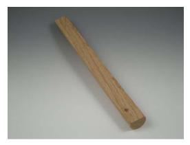
2. Using the cover plate from your coil holder carefully mark the centers of the 2 holes on the round side of the dowel. Make sure the end of the cover plate is about 1/4" in from the end of the dowel so the edge of the tee nut will not extend beyond the end of the dowel
