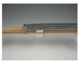
4. Position the head of the Koil Kutter over the cover plate, turn it on, and move it to the left, cutting the jump rings. Make sure to have a good grip on both the large coil holder and the Koil Kutter as there will be some resistance from the wood against the blade.
