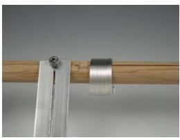
3. Apply a little burr life to the top of the coil. Attach the other end of the cover plate, and tighten the screws making sure the coil is against the stop plate.
