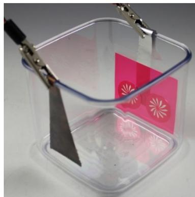
10. Lift the package out of the electrolyte and inspect the etching every 5 or 10 minutes. If a deeper etch is desired, just hang the package back into the tank and let the etching continue.
