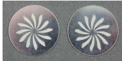
13. Punch a 1.25mm hole in each earring blank for attaching the ear wires. Be careful you don't punch the hole too close to the edge.
