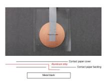
7. Hang the package on the edge of the tank by the strip of aluminum foil, and clamp it in place with the red alligator clip from the power supply. Add the electrolyte to the tank until it completely covers the metal blank, but do not allow the electrolyte to touch the aluminum strip or the alligator clip. Hang a copper cathode on the other side of the tank and connect it to the black alligator clip from the power supply.
