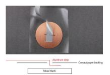
6. Cut another piece of contact paper approximately the same size as the first piece and place it on top of the first piece of contact paper. Make sure this second piece completely covers the aluminum strip from below the slit to the top edge of the first piece of contact paper.
